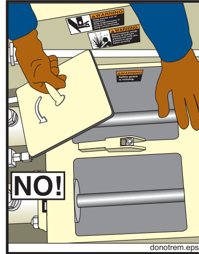
Figure 48 Do not remove the water box covers when the machine is stroking
