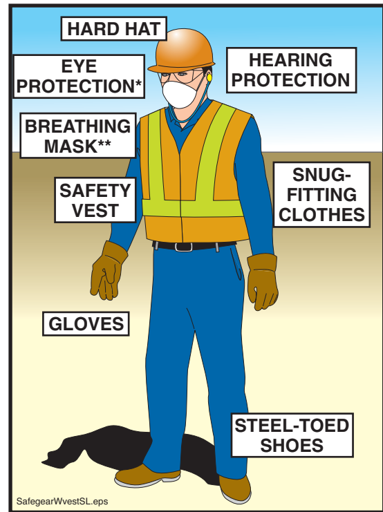
Figure 50 Wear Personal Protective Equipment (PPE)
