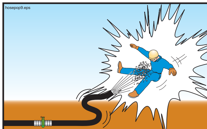
Figure 43 Remove everyone from the discharge area whenever air has been introduced into the line
