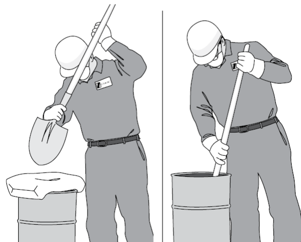
Figure 17 Mixing Slurry In Barrel
